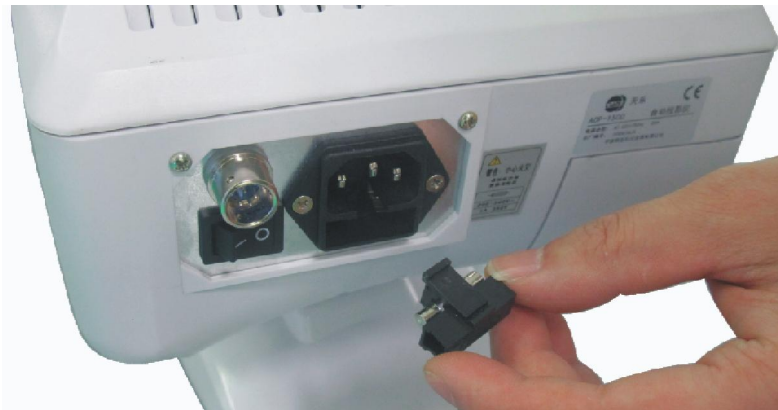
Picture 12. Replace the fuse
