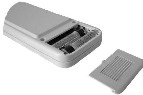
Picture 5. Insert the dry batteries
